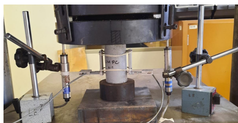
Figure 72 – Compression test setup
