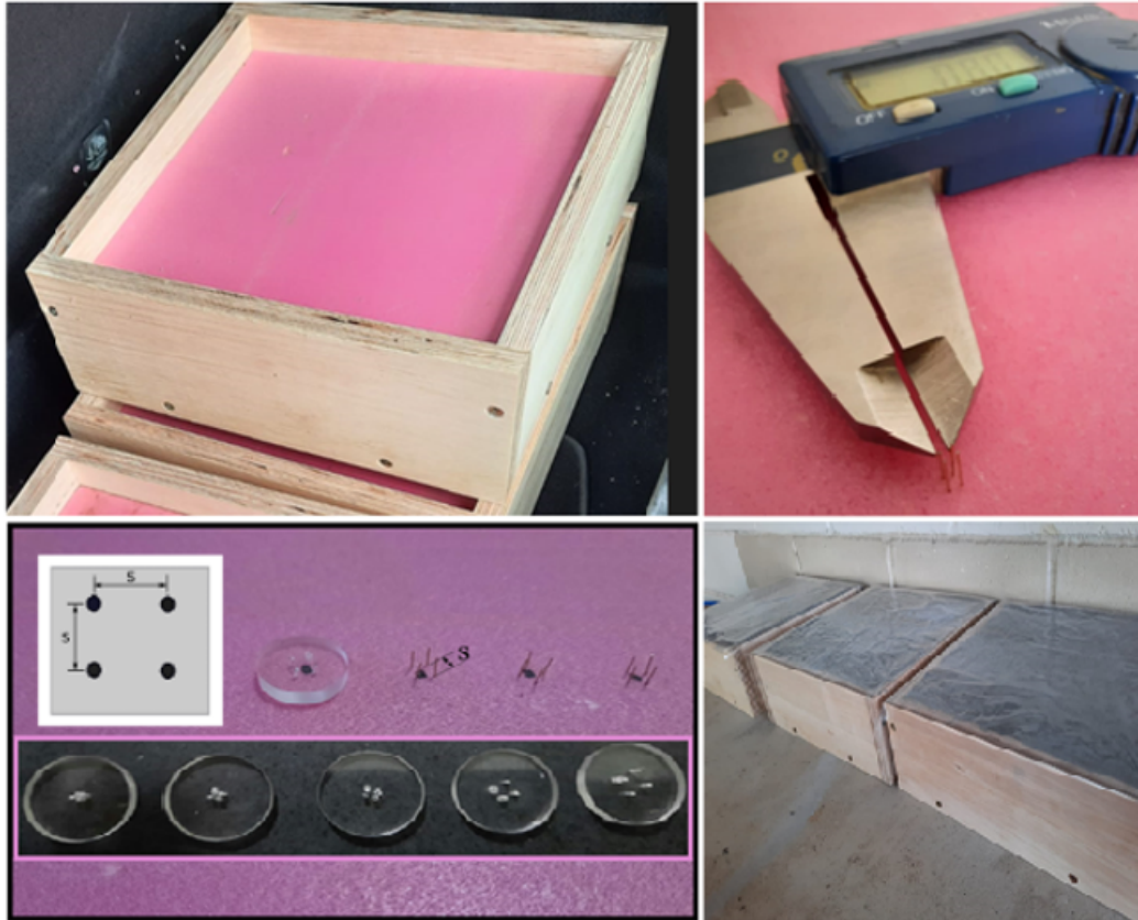
Figure 81 – Details of the fibers fixed in the styrofoam plate and anchored into the concrete plate
