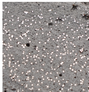
Figure 85 – Example of fiber distribution in a sample
