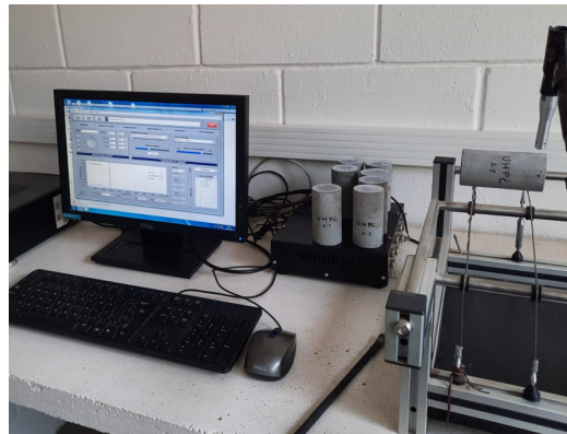
Figure 18 – Impact acoustic test configuration
