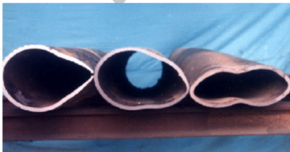
(a) Colapso (LIU et al., 2014).
