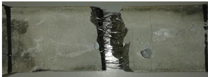
Figure 108 – Failure pattern of UHPFRC under tension
