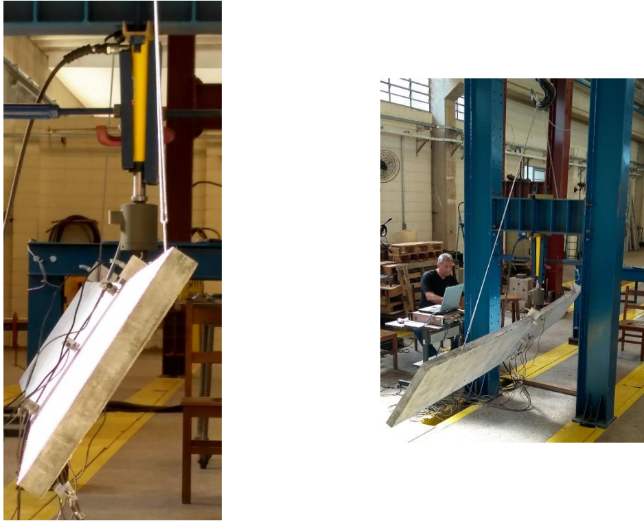
Figure 120 – Beam rotation at the end of the test
