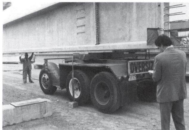
Figure 43 – Test to determine the truck roll stiffness, (MAST, 1993)
