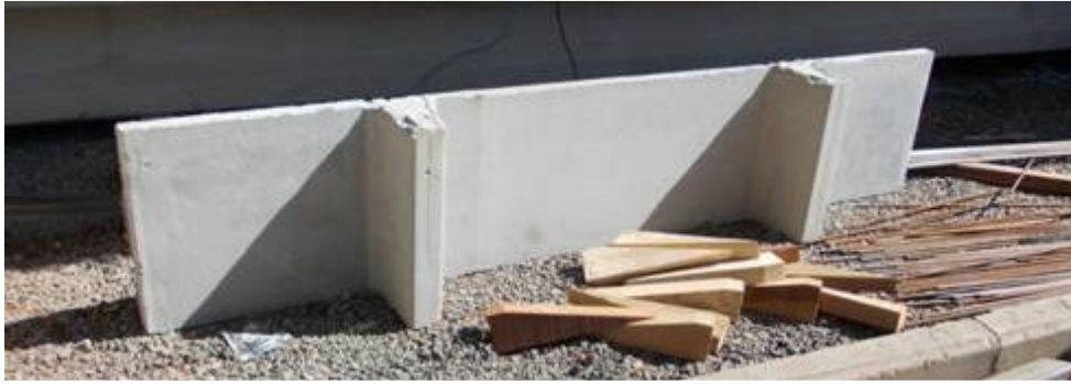
Figura 3: Painel PI de Concreto Leve com EPS (KERBAUY, 2011)
