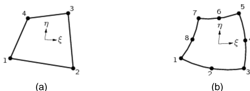
Figura 24 - Elemento Finito: (a) Q12PL e (b) CQ24P. [Diana User's Manual, Element Library (2005)].
