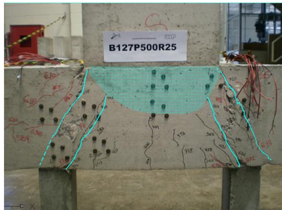
Figura 4.72 – Biela experimental B127P500R25
