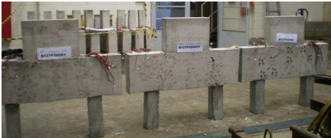
Figura 4.80 – Modelos B127P500R1, B127P500R25 e B127P500R4 após ensaio
