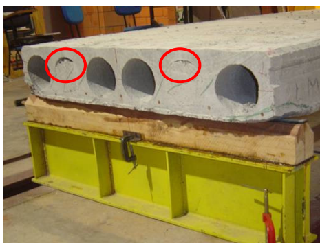
Figura 8.11: Preenchimento inadequado dos alvéolos (L5-2P-20-7D9,5-Y_C)
