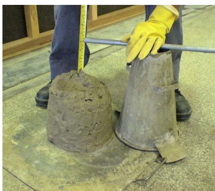
b) slump do concreto = 14cm
